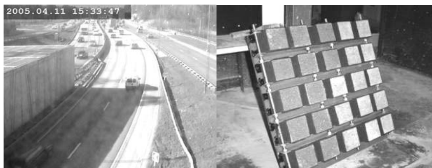
Figure 1: The picture on the left side shows a web camera photo of the traffic going into the Eugenia tunnel. The photo on the right side shows water repellent treated (light) and untreated (dark) samples before they were placed at the field exposure site in the tunnel.
