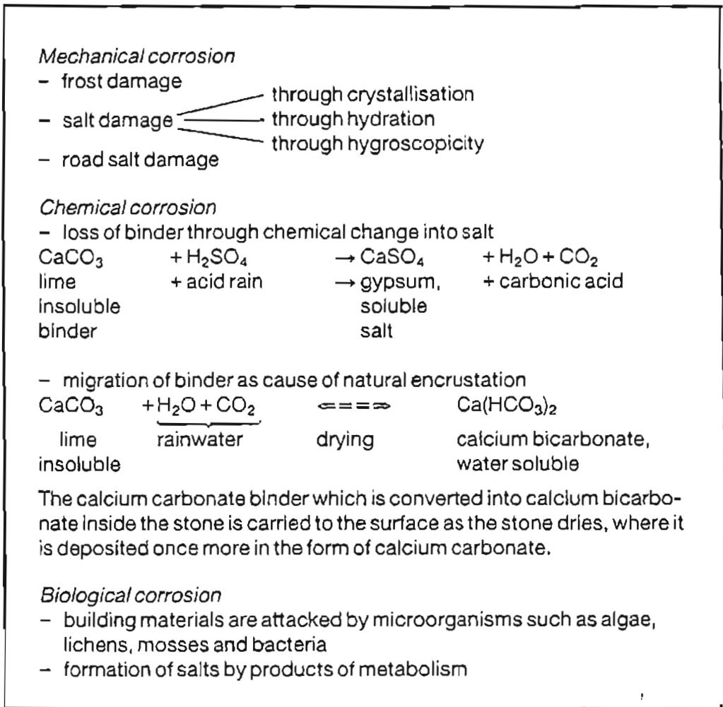
As pointed out later, the tower of Wittenberg's castle church consists mainly of porous sandstones. These stones usually weather from the inside outwards, forming crusts and reducing the surface to a thin shell:
