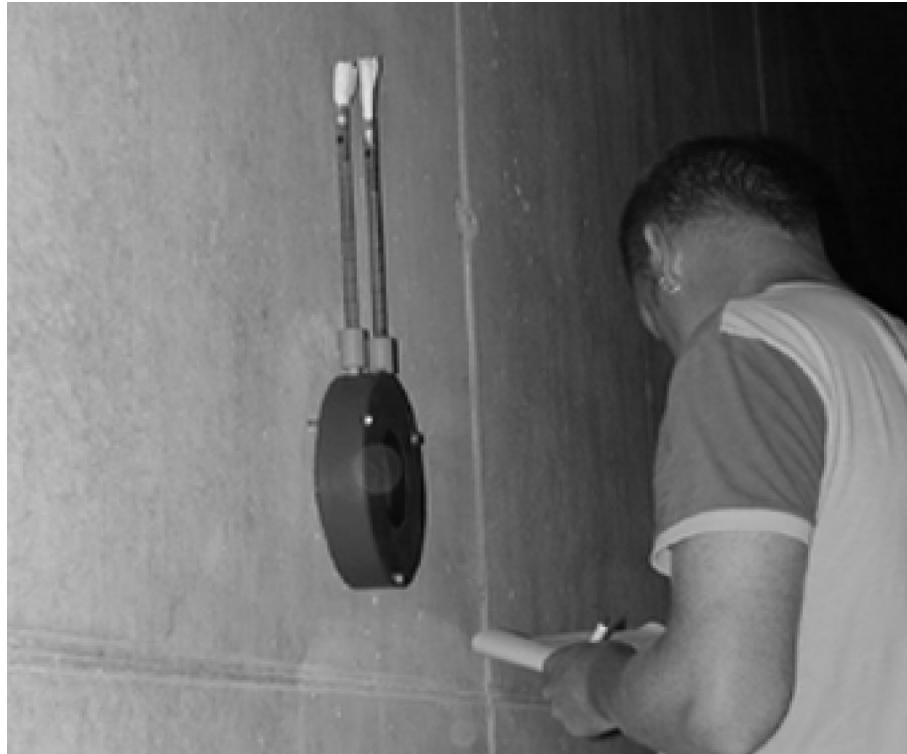
Figure 2: Preliminary investigation: Double-chamber cells for the measurement of the uptake efficiency of the water repellent by the concrete surface in the tunnel
