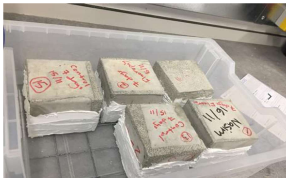
Fig.2. Testing concrete for water absorption following a modified ASTM D 6489-99 testing procedure
