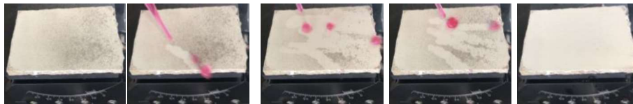
Fig.6. Snapshots of the self-cleaning process observed for the weathered coating surface tilted at a slope angle of 2^\circ after being ground with the 180-grit emery paper.
