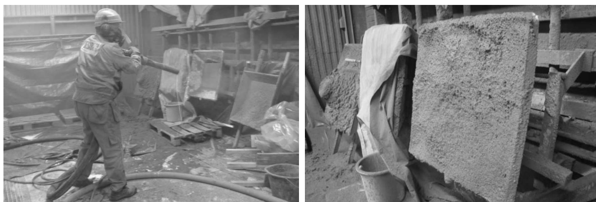
Fig. 7. During and after the spraying test. The uncovered mould contains the sprayed concrete with the agent.
