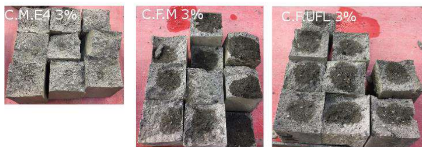
Fig.4. Bulk cement paste simple water droplet testing 2
