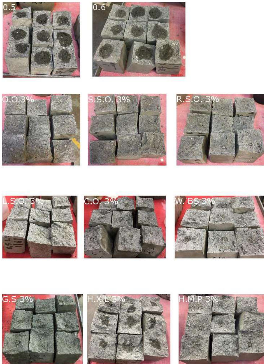
Fig.3. Bulk cement paste simple water droplet testing 1 (G.S = C.C.A)
