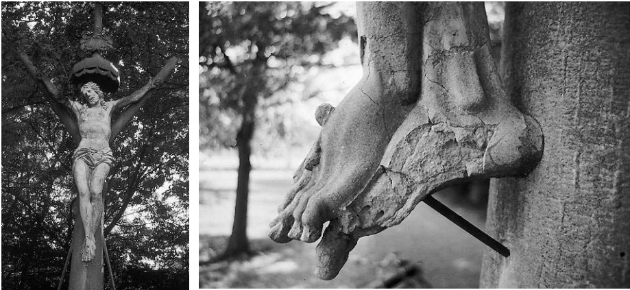
Figure 1: Left: A crucifix made of Baumberg sandstone (Münster, Germany). Right: Spalling caused by the impregnation agent that was applied (detail in the illustration on the right)
