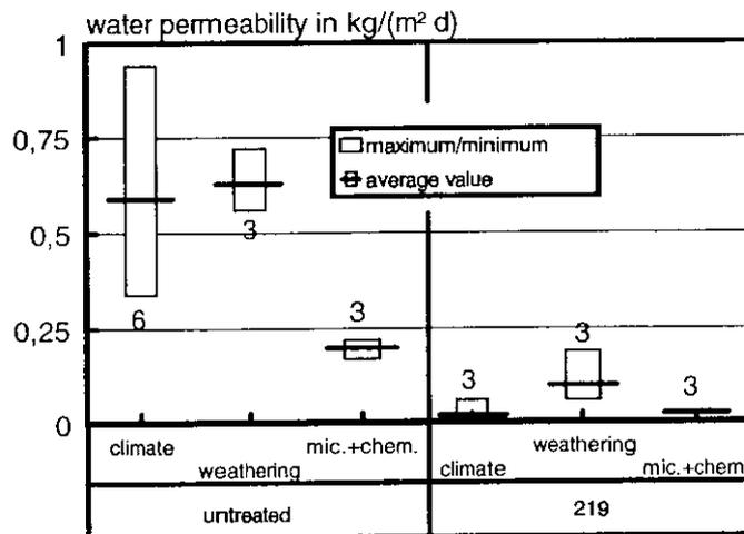
**Figure 6:** Water permeability of untreated and treated (219) Cottaer Sandstone after different stress procedures. (weathering: artificial weathering; mic.+chem.: microbiological and chemical stress)
