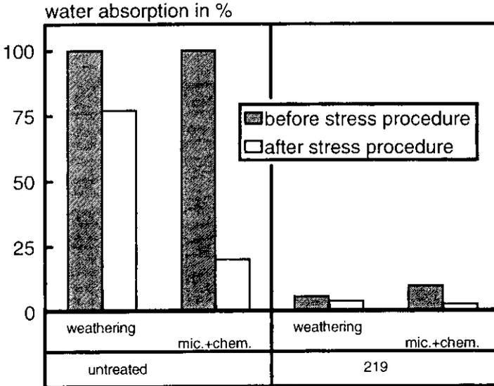
**Figure 5:** Capillary water absorption of untreated and treated (219) Cottaer Sandstone after different stress procedures. (weathering: artificial weathering; mic.+chem.: microbiological and chemical stress)
