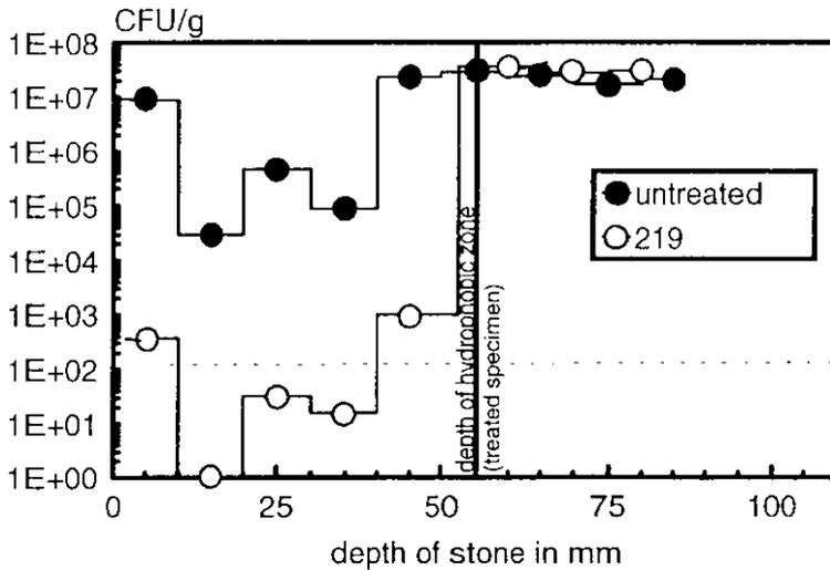
**Figure 8:** Cell numbers of chemoorganotrophic bacteria in an untreated and impregnated (219) specimen after 12 months of combined microbiological and chemical stress.
