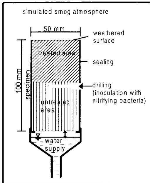
Figure 3: Test device for microbiological and chemical stress
