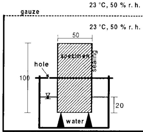
Figure 4: Test device for the determination of water permeability (dimensional unit: mm)
