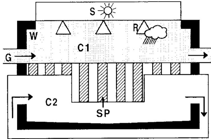
**Figure 2:** Schematic plan of the experimental system for artificial weathering
