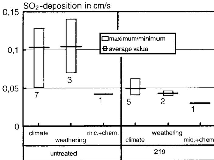
**Figure 7:** Velocity of SO<sub>2</sub>-deposition of untreated and treated (219) Cottaer Sandstone after different stress procedures. (weathering: artificial weathering; mic.+chem.: microbiological and chemical stress)
