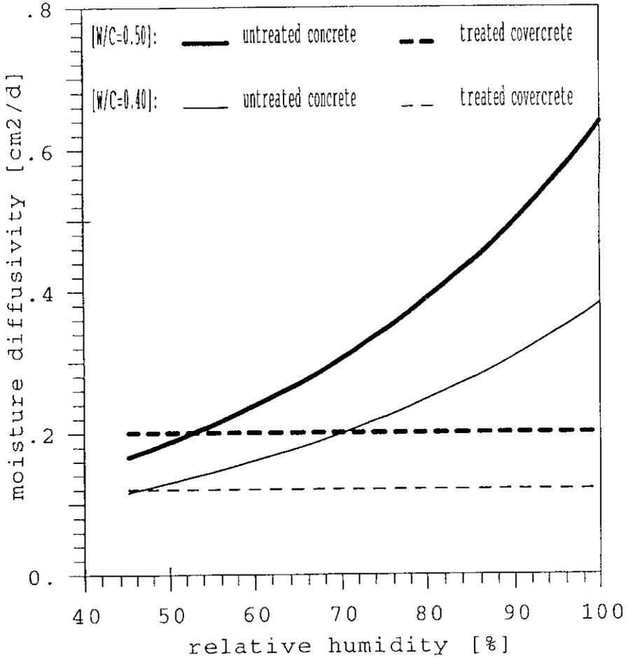
Figure 3: Diffusion coefficient for untreated and impregnated concrete
