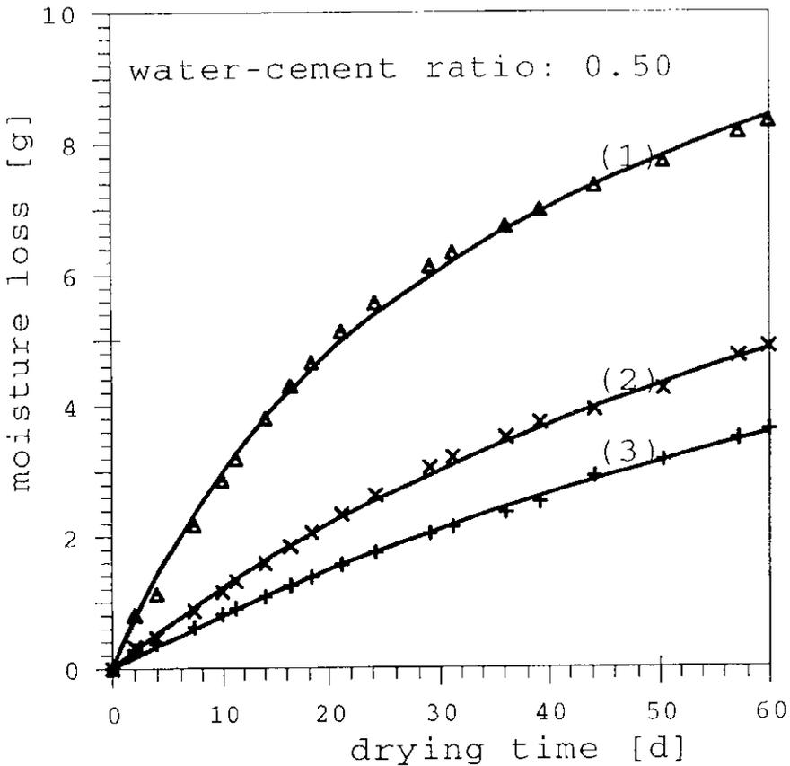
**Figure 1:** Moisture loss of untreated concrete with a water - cement ratio of 0.5 (1) and concrete with a water repellent layer of 1.5 mm (2) and 4 mm (3)
