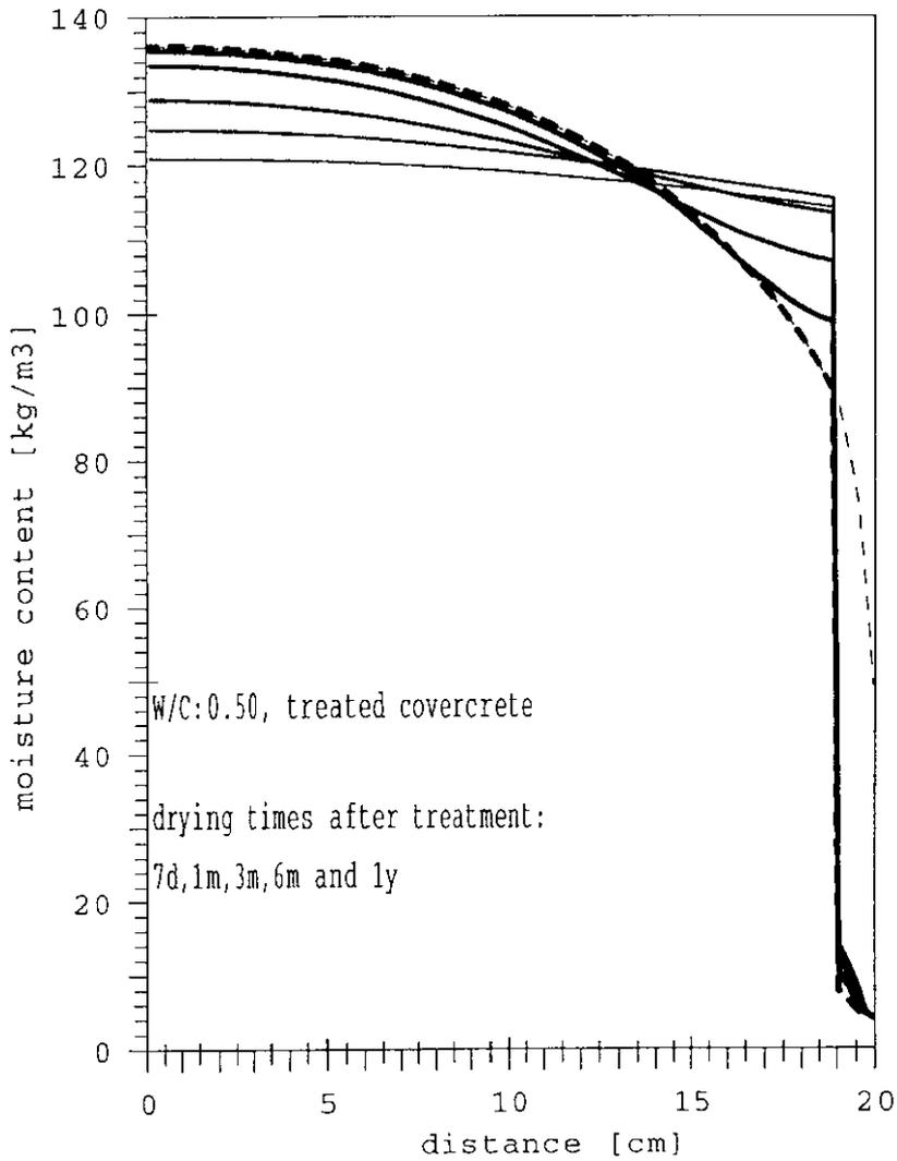
**Figure 6:** Moisture distribution in a drying concrete element (water-cement ratio=0.5) which is impregnated after 6 months of drying with a water repellent agent.
