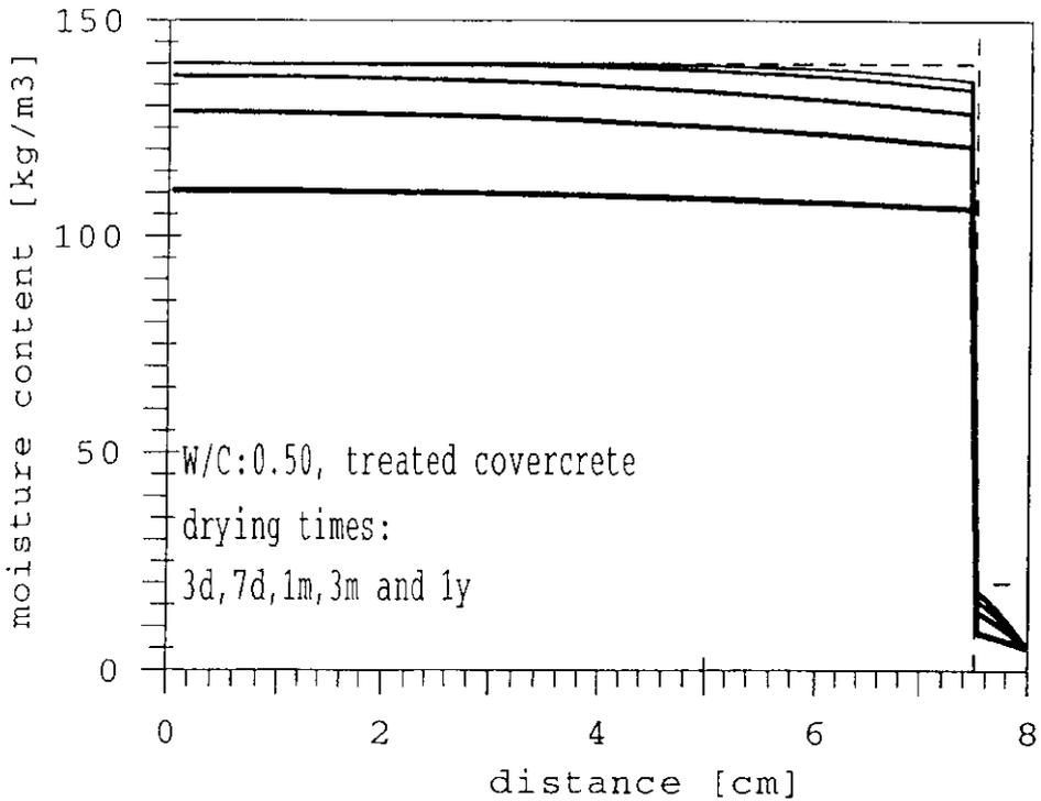
Figure 5: Moisture distribution in drying concrete (water-cement ratio = 0.5) with an impregnated layer of 5 mm thickness after 5 selected durations of drying.
