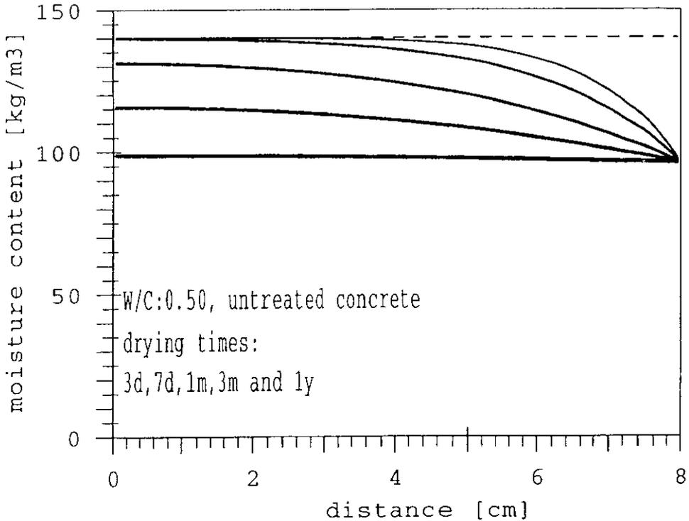
Figure 4: Moisture distribution in drying concrete with a water-cement ratio of 0.5 after 5 selected durations of drying.
