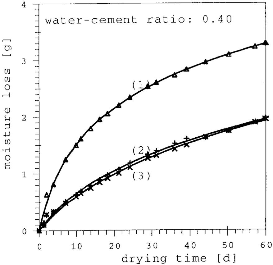
Figure 2: Moisture loss of untreated concrete with a water - cement ratio of 0.4 (1) and concrete with a water repellent layer of 1.0 mm (2) and 1.1 mm (3)
